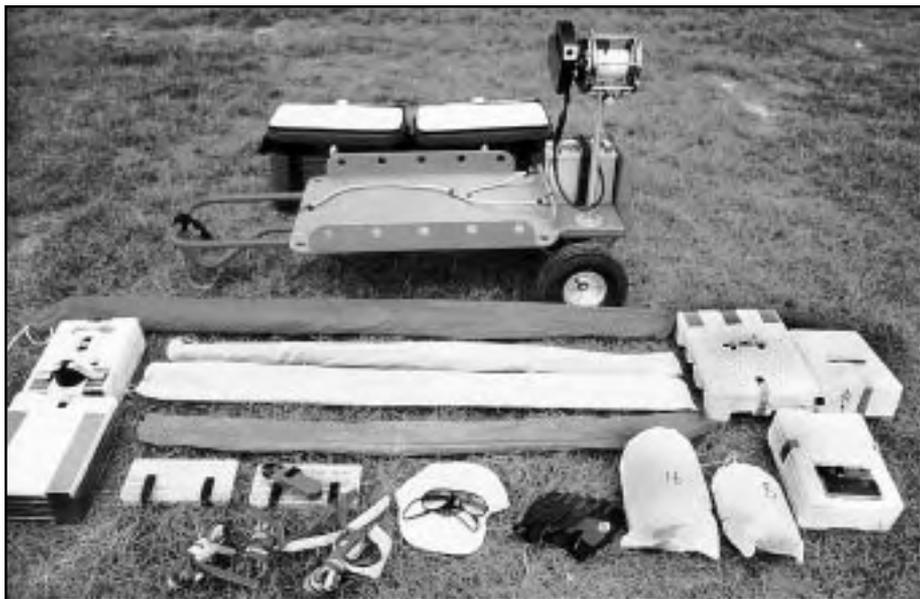
A platform or bed, made of 1/2" plywood, is attached to the top side of the hand truck's frame. The two containers carried on the bed are insulated fabric coolers, with zipper-closure tops and semi-rigid plastic liners.
