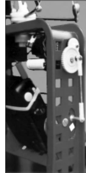
This installation allows me to control tilt with an up-stick movement, using a crankshaft [left] to convert the endless rotation to 90 degrees of tilt, and down-stick to close the switch and click the electric shutter.
